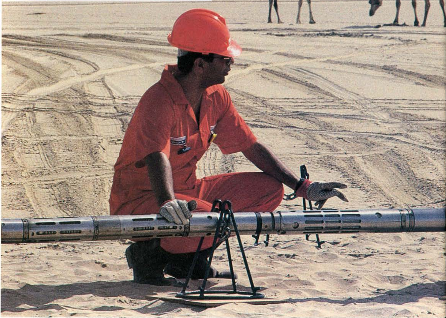
● PREPARING THE DSI TOOL FOR LOGGING A WELL IN ABU DHABI ARE GENERAL FIELD ENGINEERS TAMER FAWZY, LEFT, AND RAMIRO APONTE.
