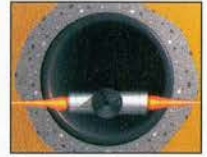
Seen from above, Pivot Gun® charges deployed and fired. A jet from the detonation penetrates the steel casing, cement and rock formation, permitting hydrocarbons to flow into the well.
