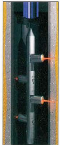
Once the Pivot Gun is lowered to the proper depth, charges swing out from the body of the tool. This design allows more powerful charges to be built into a gun of small diameter.
