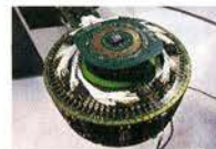
Chip mounted in the center of the test head, ready for testing.
