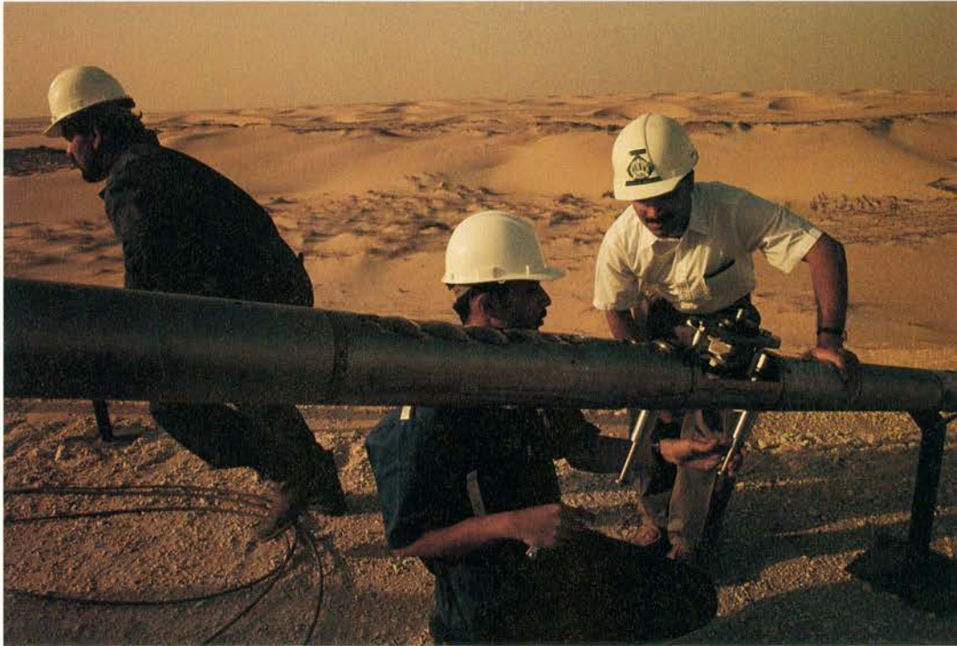
The MDT Modular Formation Dynamics Tester is one of many high-technology logging tools made accessible to a wide range of markets by the MAXIS Express system. Near Dhahran, Saudi Arabia, Operator Javed Nazir, left, unloads equipment while Engineer Yasser Mufti, middle, reviews functions of the MDT tool with Aramco Supervisor Abdullah Al-Daalouj. The MDT tool collects fluid samples from rock formations and measures how easily oil or gas will flow into a well.
