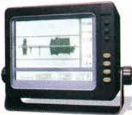
The TIM screen keeps the engineer informed about tubing fatigue.
