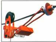
Tubing condition on the job is measured by the TIM® Tubing Integrity Monitor.
