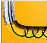
As tubing buckles in the well, friction may increase enough to stop progress of the tubing.
