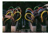
High-speed electrical cables link the test head with the main computing engine.
