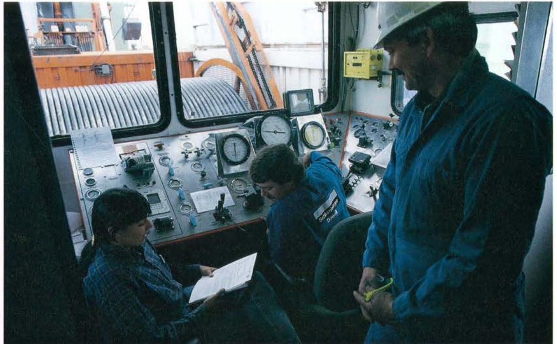
Wireline logging with coiled tubing in Prudhoe Bay, Alaska. Left, ARCO Engineer Jennifer Julian compares notes with Paul Perius of Dowell, seated, and Gerry Bailey of Schlumberger Wireline. In wells highly deviated from vertical, coiled tubing allows pushing sensors down to the depth of interest.
