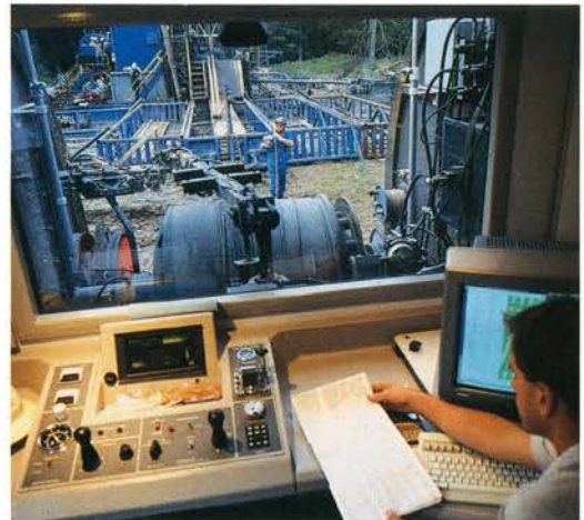
Senior Operator Dave Whiteley, center, prepares sensors to make measurements in a well in Wise County, Texas, while General Field Engineer Harvin Broughton, foreground, prepares the onboard computer that controls the sensors and records their measurements. The layout of the logging unit increases productivity of field operations, allowing the engineer to simultaneously control the computer and the winch that moves sensors in and out of the well.
