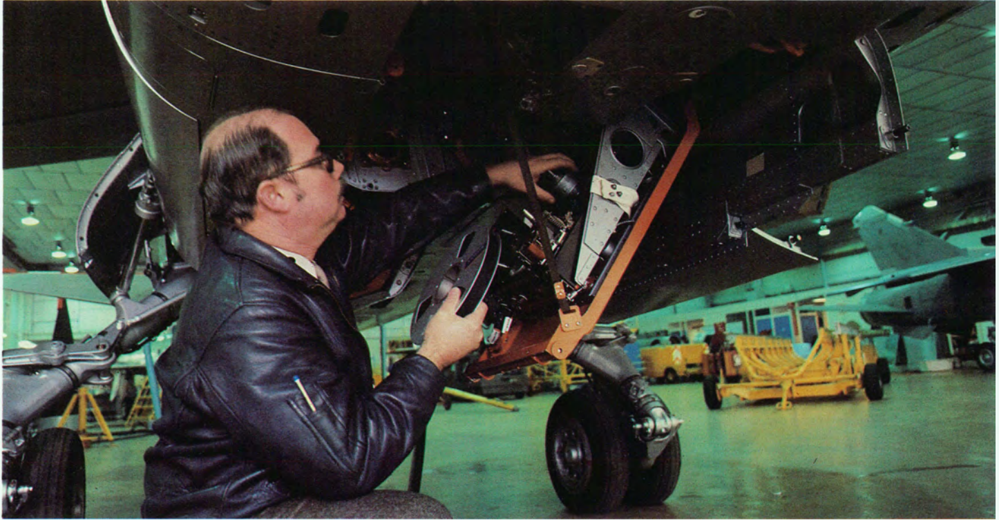
This Enertec flight-data recorder, being installed in a Mirage jet fighter at the Brétigny Flight Test Center in France, stores information on the aircraft performance during missions.
