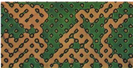
A 6 mm x 1 mm section of "simulated" rock used in studies of fluid flow in formations. Oil (yellow) is invading the water-filled (green) interstices. Often water or oil is trapped by this finger-like displacement process.
