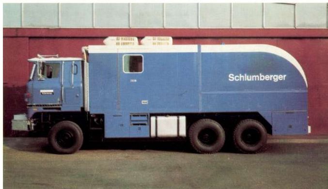
The Schlumberger CSU Wireline Logging Truck
