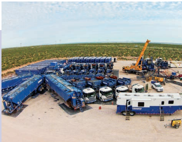
Well Services pressure pumping equipment deployed in a spread on a wellsite in Neuquen, Argentina prior to a hydraulic fracture operation on a shale gas well in the Vaca Muerta formation.
