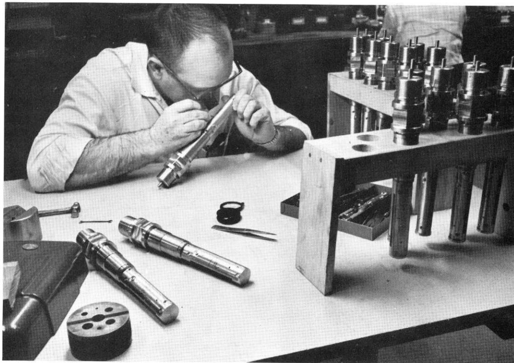
Pressure measuring and recording instruments being checked at Johnston Testers.
