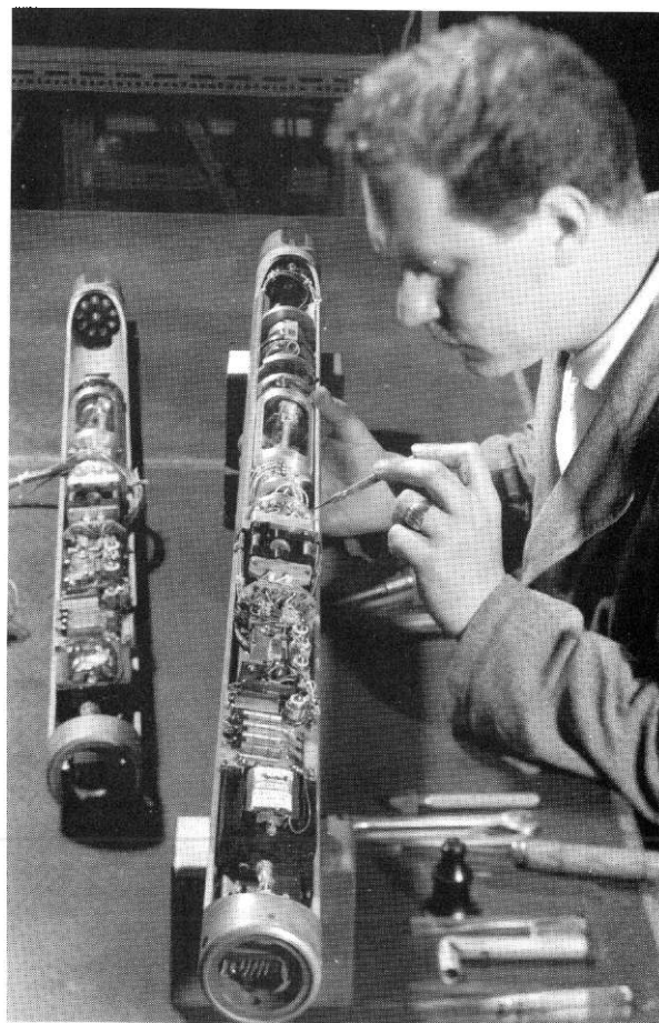
Pressure measuring and recording instruments being checked at Johnston Testers.
