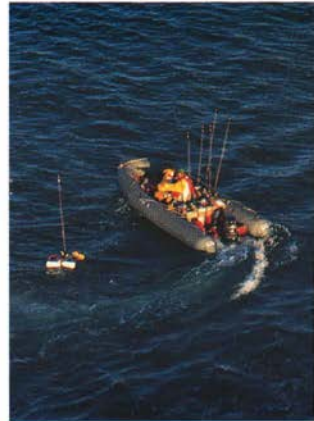
The Digiseis-FLX system assists with the search for hydrocarbons in nearshore Southern California. Data acquisition units connected to receivers pick up acoustic pulses and transmit them to a central computer. Use of radiotelemetry, instead of transmission by cable, allows quick and flexible deployment of receivers, reducing survey time and resulting in less disturbance to sensitive nearshore environments.
